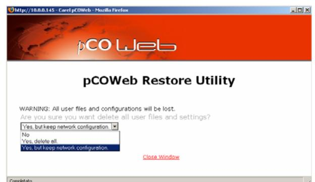
Figure 8.i - Restoring *pCOWeb* to the default situation
