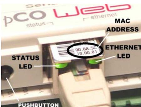
Figure 2.e - MAC address and indicator LEDs
