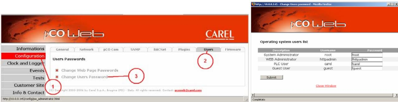
Figure 8.y – Changing the password for the operating system access Usernames
