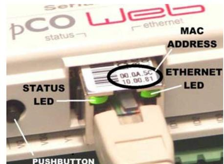
Figure 1.b - MAC address and indicator LEDs
