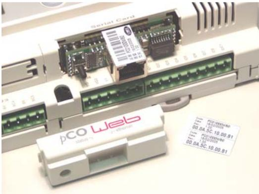
Figure 2.c – Inserting *pCOWeb* in the *pCO* controller
