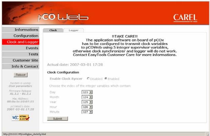
Figure 8.m - Setting clock synchronisation
