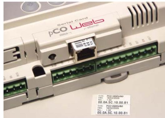
Figure 2.d – Securing *pCOWeb* with the cover
