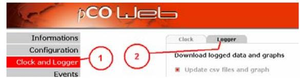
Figure 5.a - Opening the Logger and Graph settings
