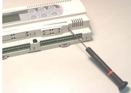
Figure 2.b – Removing the cover from the *pCO* controller
