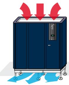
Downflow unit installed on access floor.
