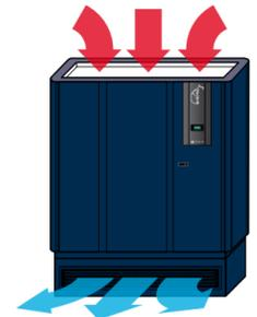
Downflow unit with enclosed floor stand and front discharge.
