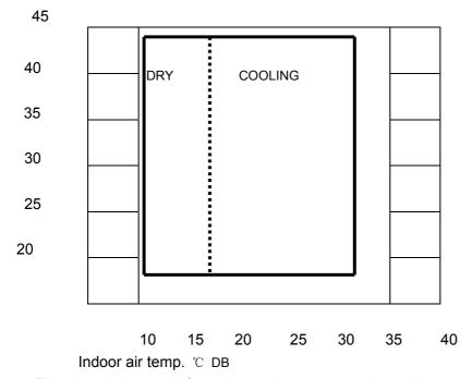
Note: The chart is the result from the continuous operation under constant air temperature conditions. However, excludes the initial pull-down stage.
