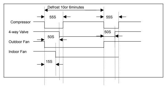
Remark: when the evaporator pipe sensor temp. more than TE16, The indoor fan start to run.
