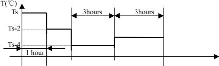
As shown in the above diagram, after running for 1 hour under refrigerating mode and dehumidification mode, the setting temperature will increase 1°C; after another 1 hour, it will increase 1°C again, and after 6 hours, it will cease; after running for 1 hour under heating mode, the setting temperature will decrease 2°C, after another 1 hour, it will decrease the 2°C again, and after 3 hours, it will increase  $1^{\circ}$ C, and after other 3 hours, it will cease.
