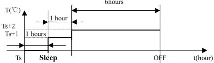
After setting the sleeping function, the heating mode will run as per the following rules:
