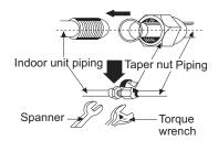
NOTE: Connect the connection pipe to indoor unit at first and then to outdoor unit. Handle pi-ping bending with care. Do not damage the connection pipe. Ensure that the joint nut is tightened firmly, otherwise, it may cause leakage.
