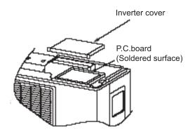
(2)As shown below,connect the discharge resistance(approx.100Ω20W)or plug of the sold ering iron to voltage between + - terminals of the electrolytic capacitor (test3 "D" and "E" point) on PC Board for 30s, and then peformedischarging.
