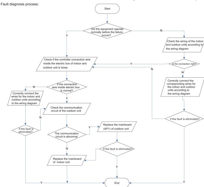
Detection process of outdoor communication circuit (refer to the outdoor key detection points)
