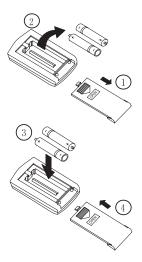
Sketch map for replacing batteries
