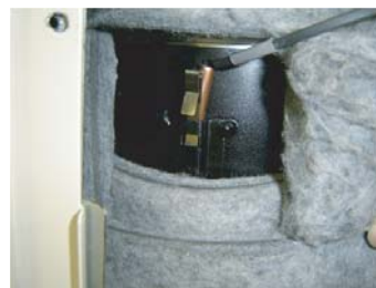
Remove the THERMISTOR SPRING with the THERMISTOR (Compressor temp.)
