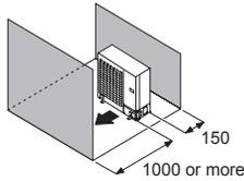
**When an obstruction is present also in the upward area** (Unit : mm)
