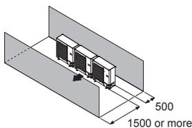
**When an obstruction is present also in the upward area** (Unit: mm)
