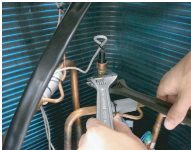
Remove the PRESSURE SENSOR with wrench.
